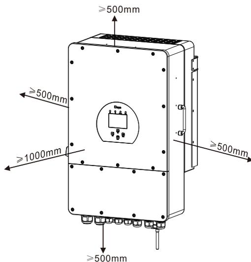
For proper air circulation to dissipate heat, allow a clearance of approx. 50cm to the side and approx. 50cm above and below the unit. And 100cm to the front.
